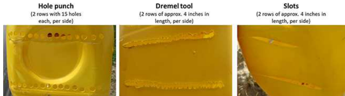
FIGURE 3-B. The three types of entrance holes for cucumber beetles that were evaluated. The entire surface area is similar across opening types.
